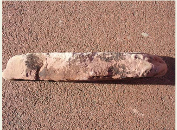
Worn edge surface on left, fresh surface in middle
